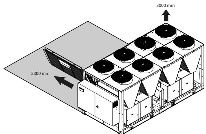
C2 = Minimum technical space, to be ensured in order for the chiller to work properly and for possible maintenance.
